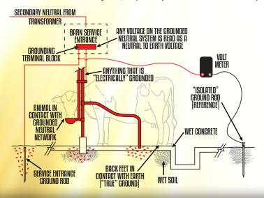
come into contact with anything grounded. This includes metal stanchions, stainless steel milk lines, or anything metallic. Cows can sense a voltage of around 1.0 volt to ground. Voltage should be 0.5 volts or less on a farm site.
